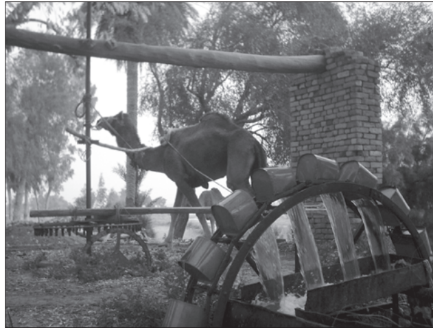
The Persian wheel has been used to supply water for irrigation in Egypt, the Mediterranean countries, India and China.
